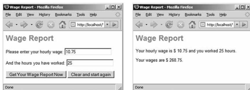
Figure 2-5: Client/Server Example using HTML and PHP
